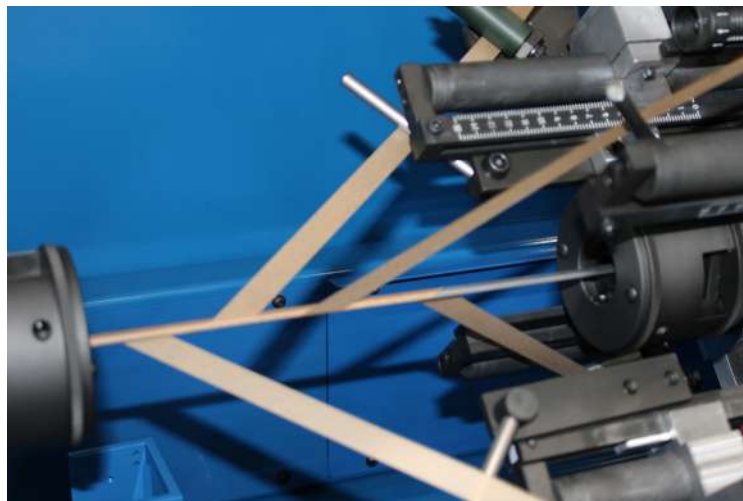
4 Pad Head, ideal for high insulation build applications. Head speeds up to 1000 RPM
