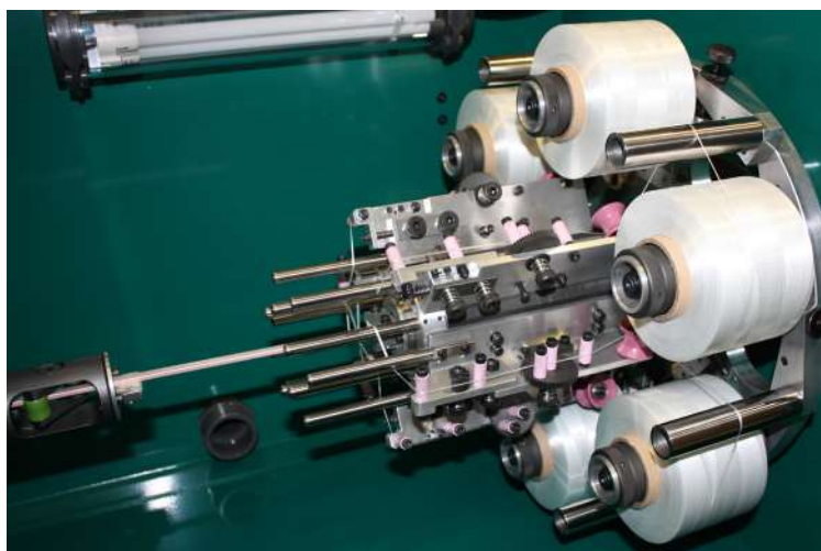
6 Bobbin Glass Taping Head being used for applying glass yarn
