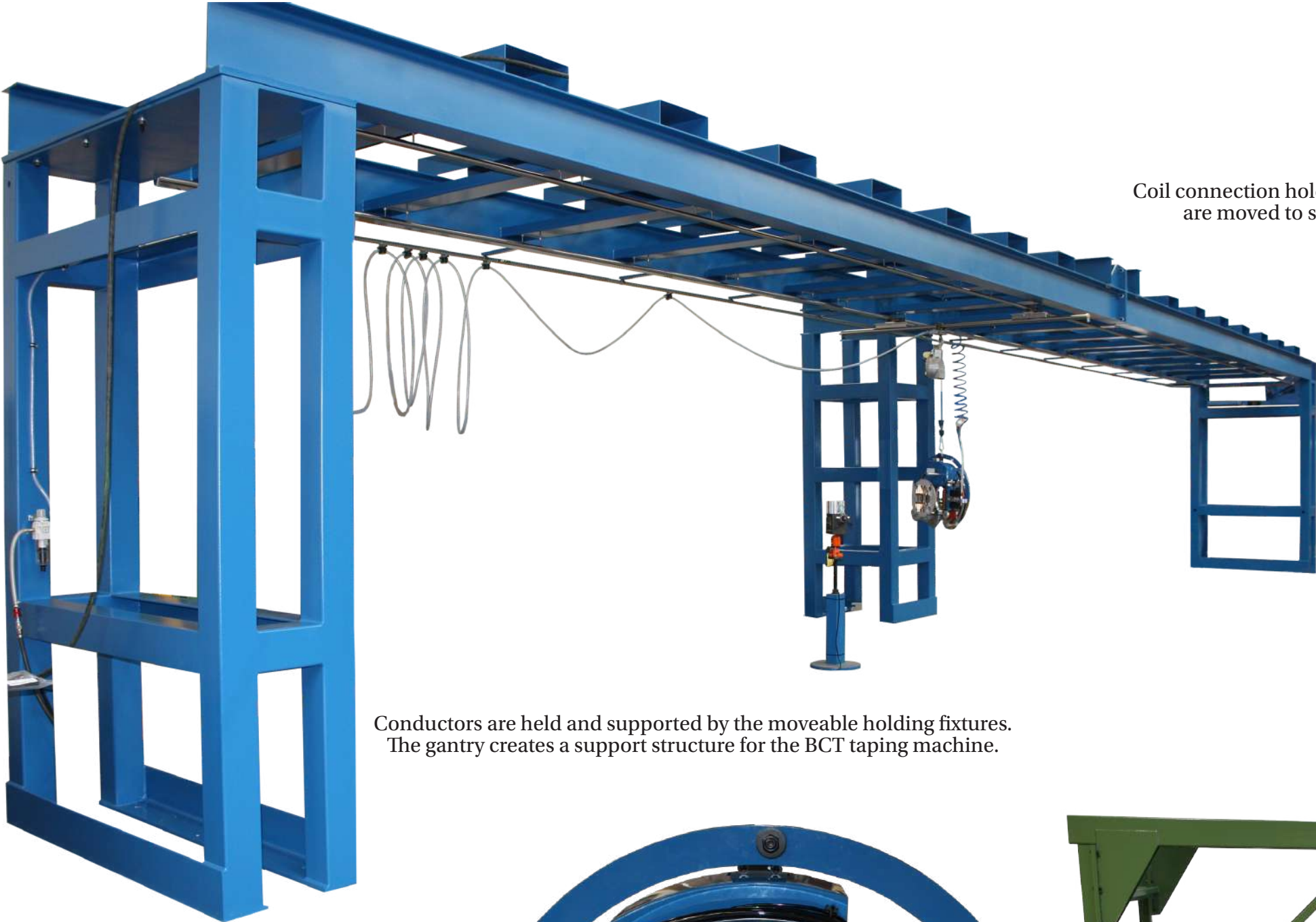
18m long x 4m wide BCT Taping Machine Gantry
