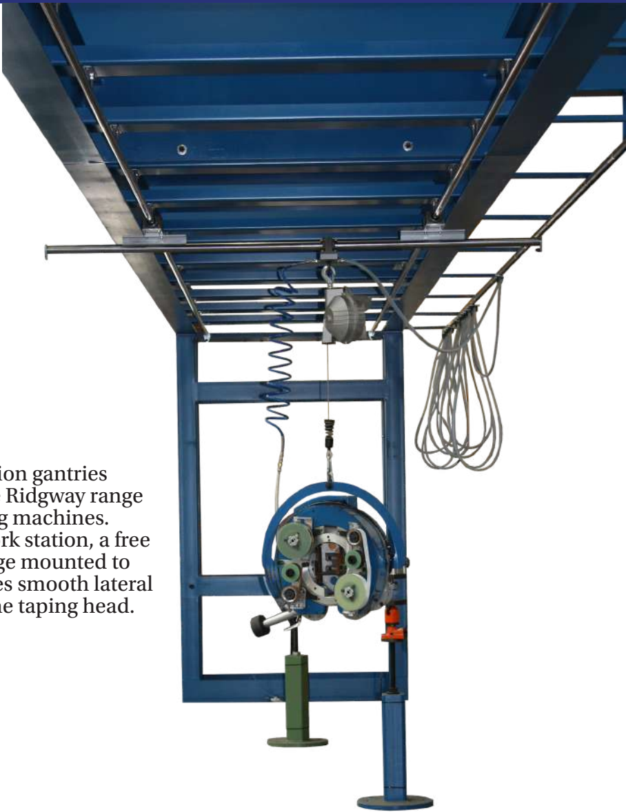
9m long x 3m wide BCT Taping Machine Gantry
