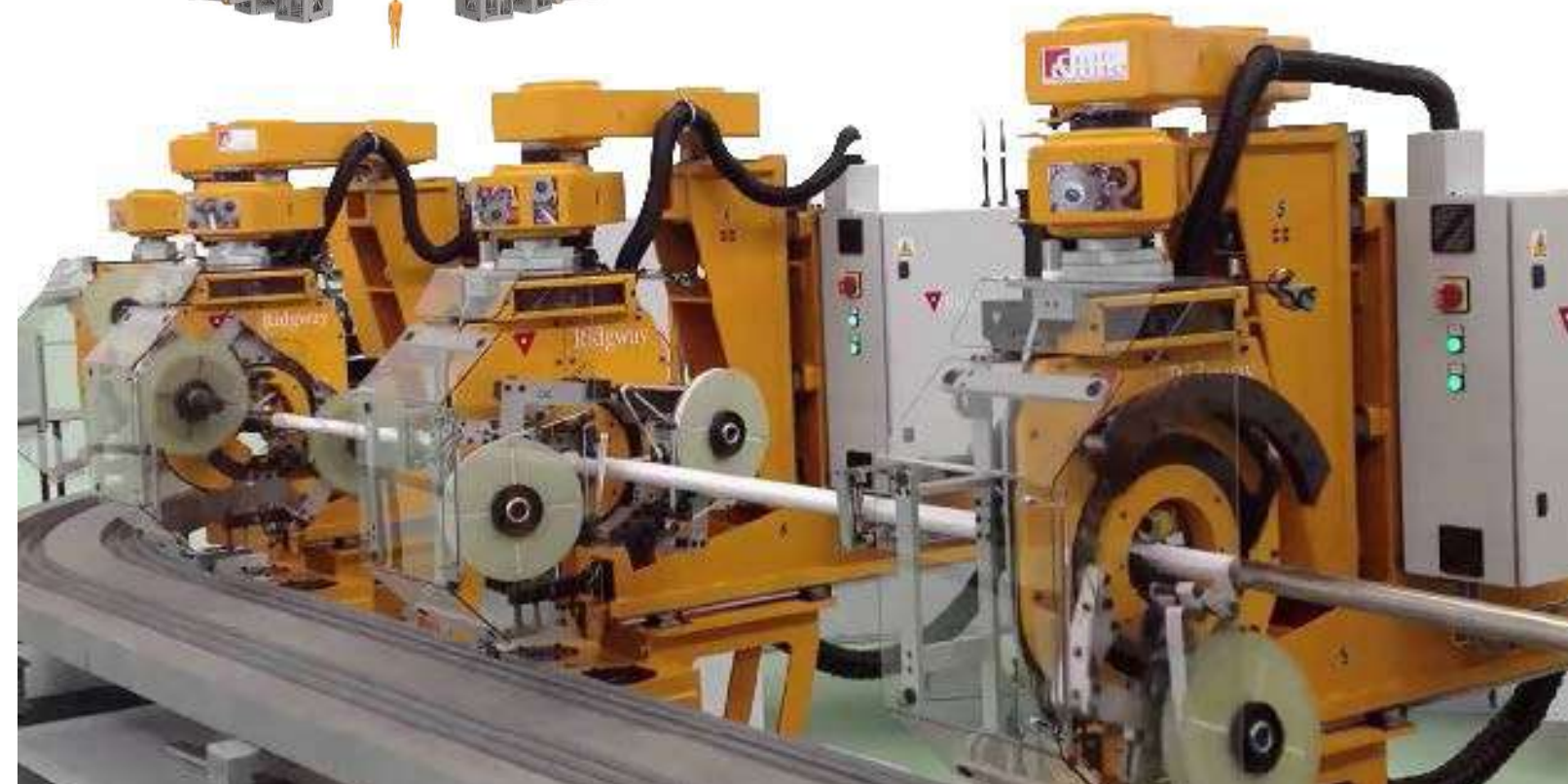
Poloidal Field coil wrapping machine supplied to Sea Alp. Coils were up to 26m outside diameter.
