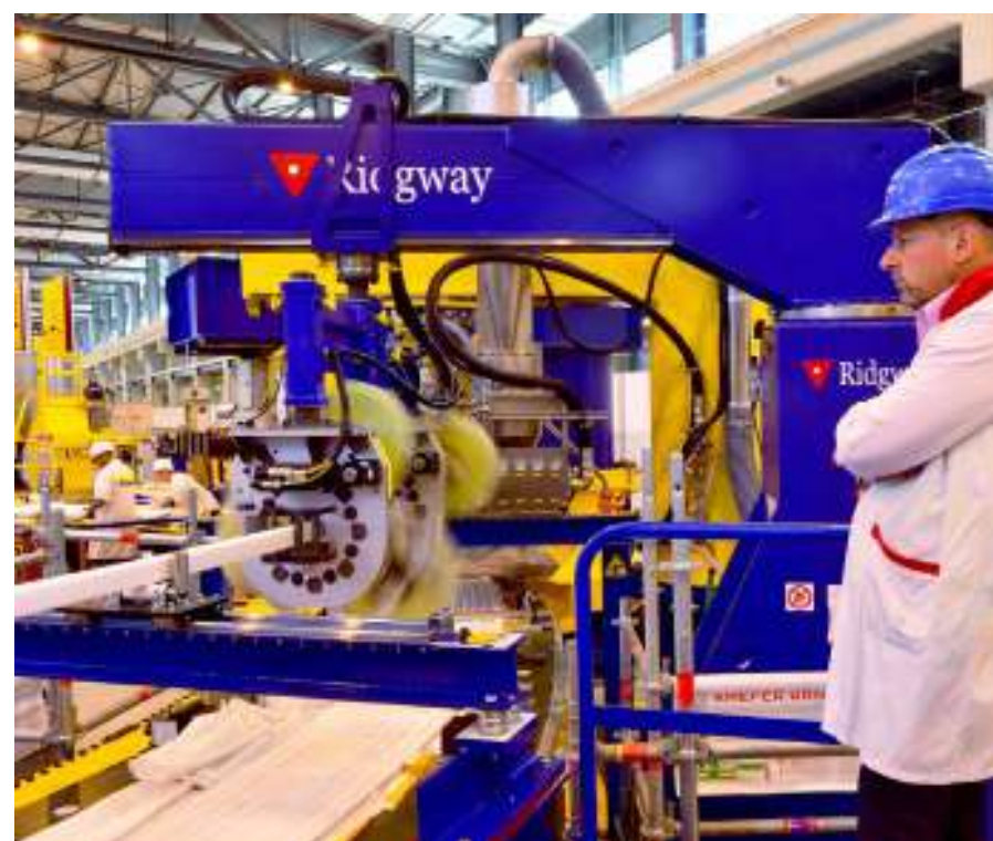
Ridgway supplied the insulation wrapping machines for the Central Solenoid, Poloidal Field and the Toroidal field coils for the ITER Tokamak. Typically the coils were wrapped with Kapton and glass tapes.
