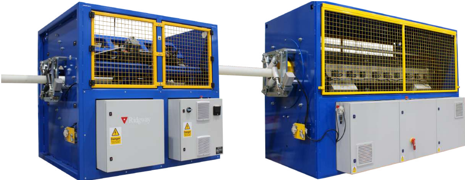
The 4 track caterpillars are self-centring to accommodate a range of pipe diameters. They pull the pipe through the line at a controlled speed. This provides a speed signal that the tape heads synchronise to ensuring accurate tape wrapping.
